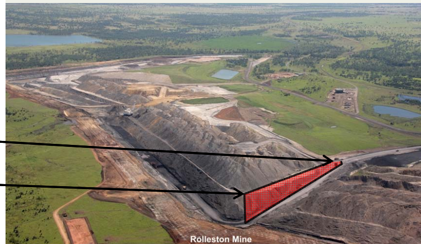
Rolleston Mine, Queensland – example of an 8Mtpa dragline operation similar to that under consideration for Sese Stage 3
